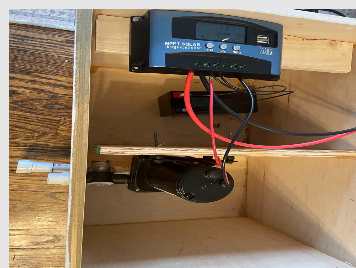
Fig 6. The images depict the solar pump that I built, it shows the outside box, pump components, the electric components, and the hinged lid (left: outside view; right: inside view).
